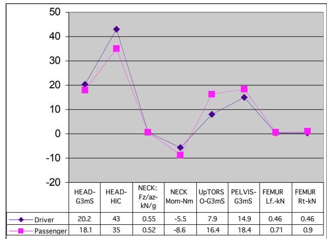
Figure 25. Comparison of Injury loads, rear end crash test.
