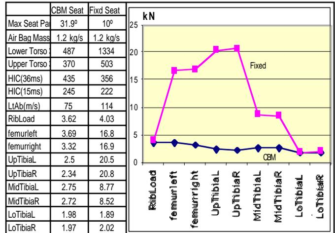
Figure 15: Peak Loads Unbelted - CBM vs Fixed
