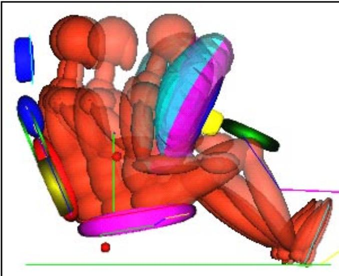
Figure 14: Fixed Seat - Unbelted Crash Kinematics.
