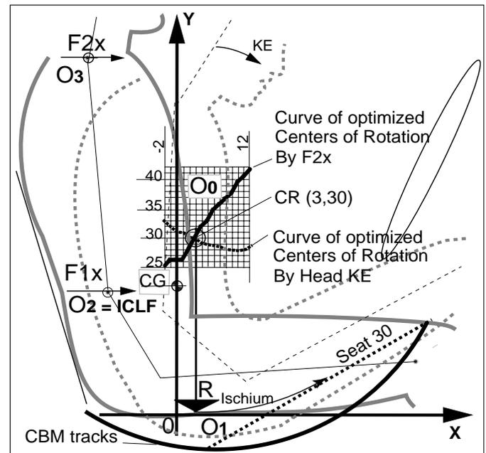
Figure 6: Dynamic Model Setup - Optimized Center.
