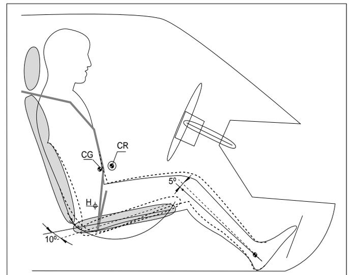
Figure 4: Automatic Lumbar & Seat Tilt Adjustment
