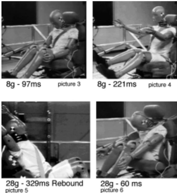
Figure 5: 8 and 28 g test at peak and rebound
