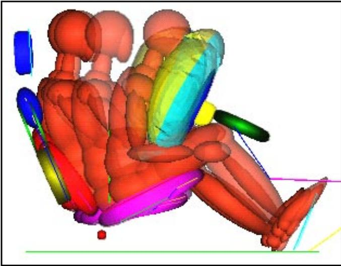
Figure 13: CBM Seat - Unbelted Crash Kinematics
